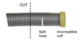
Hose Cutting. If your existing cuff is not compatible with new handle, the cuff is damaged or if the hose is split (near the handle) cut the hose behind the existing cuff using a sharp bladed knife. Ensure the cut is perpendicular (not angled). Then go to step 2.
