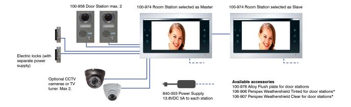
Door station/s to Room Station/s minimum wiring requirements: 4 core screened cable (100-960) + RG59 coax, star wired to master. In some installations the 100-958 Video Door Station may have audio feedback when used with a weathershield. A simple modification to the microphone gain is available - please ask when ordering.
