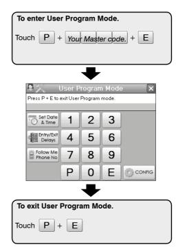
The panel will automatically exit Program Mode if the keypad is inactive for 4 minutes.
