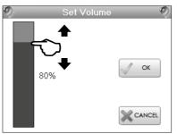
Slide your finger along the Volume slider to adjust the touch screen beep volume from 1% to 100%. The volume cannot be set to zero.
